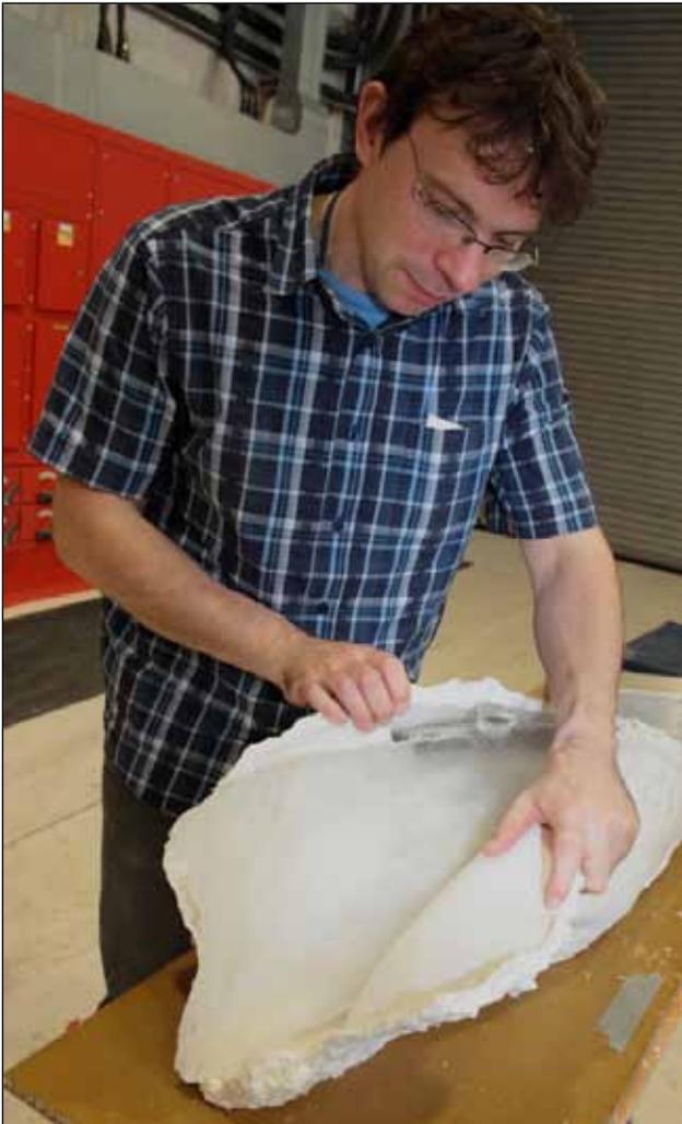
**Fig. 9:** Crystal Clear 204 cast of new stern section removed from its mould.
